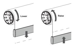
Warning: Do NOT raise it where the bottom rail will hit the fabric roll. This could damage the fabric over time.
