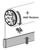
• For Reverse Roll Shades, the Right Wheel will adjust the spring tension.
