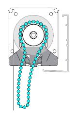
SL10 & SL15: Attach Chain Diverter Cover
