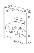
Align Clutch end first, swing assembly to bracket
