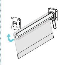
Ensure Clutch Hooks engage Bracket
