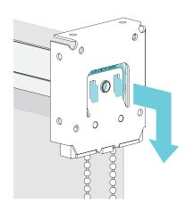
Align the chain in the diverter (SAME POSITION FOR ALL CLUTCHES)
