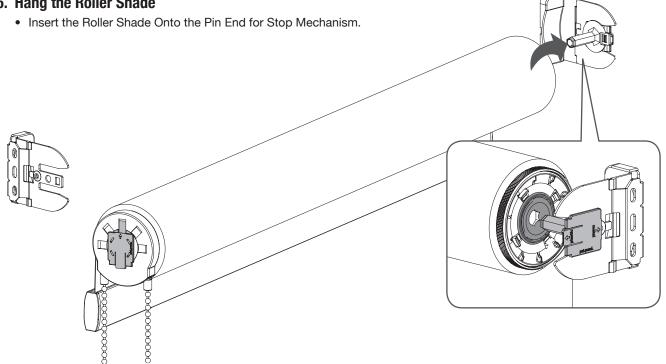
• Align the Arrow with the direction of the bracket.
