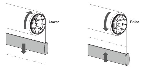
Warning: Do NOT raise it where the bottom rail will hit the fabric roll. This could damage the fabric over time.
