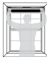
1.2 Use a pencil to mark where you will need to install the mounting brackets. If you're installing an inside mount shade, align the brackets with the front edge of the window trim, 2 inches in from each side of the window.
