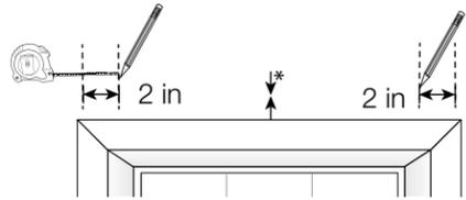
\*NOTE: Shades wider than 45 inches (vinyl headrail) or 48 inches (aluminum headrail) will need a third bracket (3). Install this bracket 2 inches to the left of the drive (the box in the middle of the headrail).
