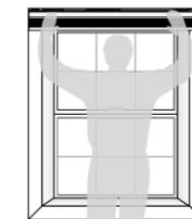
2.2 Then use a pencil to mark where you'll need to install the mounting brackets, 2 inches in from the marks you made in step 2.1.
