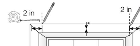
\*NOTE: Shades wider than 45 inches (vinyl headrail) or 48 inches (aluminum headrail) will need a third bracket (3). Install this bracket 2 inches to the left of the drive (the box in the middle of the headrail).
