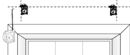
**3.4** Using the brackets as a guide, mark hole locations and then pre-drill holes for the screws. Place a spacer behind each bracket (to ensure that the shade clears the window trim).
