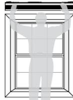
**3.2** Use a pencil to mark where you will need to install the mounting brackets, 2 inches in from the marks you made in step 3.1.
