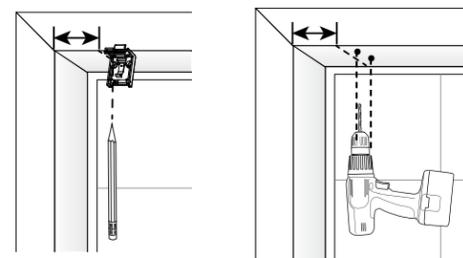
1.4 Install the mounting brackets, using the provided screws. Place each bracket flush against the front of the window frame and, using the cordless drill, drive each screw through the holes in the top of the bracket.
