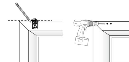
2.4 Install the mounting brackets using the provided screws. Place each bracket flush against the trim (using spacers behind brackets if needed) and using the cordless drill, drive each screw through the holes in the bracket.
