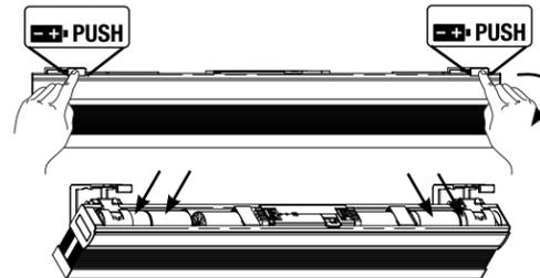
**4** Remove all of the batteries from each side of the tray, beginning with the battery that's closest to the middle of the headrail. After you have taken that battery out, slide the next battery over and remove it. Now you can insert the new batteries, following steps 1 and 2 above.
