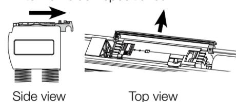
1.6 Install the shade in the brackets. Holding the shade in both hands, tilt the top of the shade slightly away from you and hook the front edge into the brackets behind the battery release tabs. Then gently tilt the shade down and press the bottom of the headrail until you hear it click into place.
