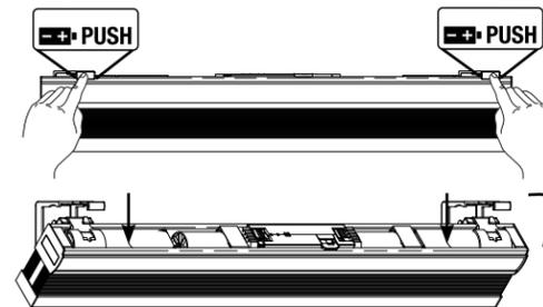
**2** Install the batteries as indicated in the battery trays (so the + / - signs match). Make sure the batteries are fully inserted in the trays.
