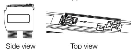
Move it out to the operating position behind the headrail, and snap it into place.
