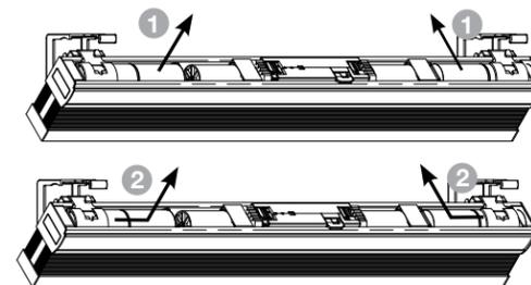
\*3-year battery life based on 2 up and 2 down movements per day assuming a 3 ft. wide by 5 ft. tall shade using light-filtering fabric. Battery life can vary between 2 to 5 years depending on shade size and fabric selection.
