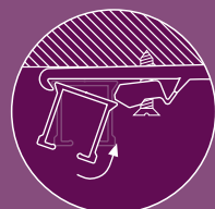
Easy installation click - position - tighten
